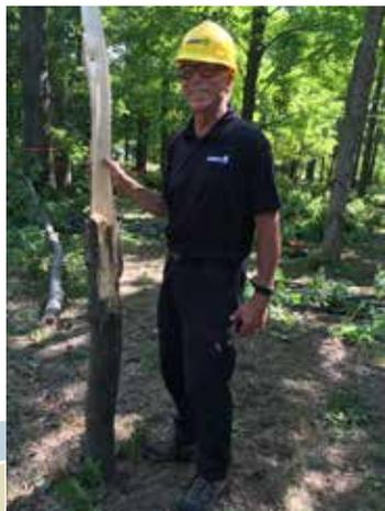
In 2016, Adolfo Sanchez of Guadalajara, Mexico carried pull testing to the next level. Winching branches in two directions simultaneously, he documented the effects of torsional loading. “The 45-degree angle of failure indicates both forces at work. We
